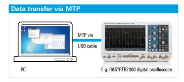
Connect the USB type B device port on the rear of the oscilloscope to a PC USB host port and use the following features:
