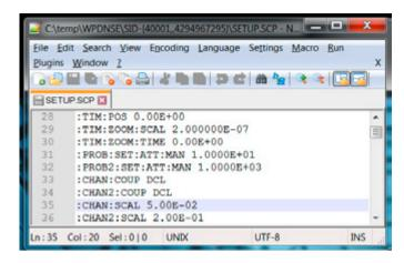
If you cannot find the user manual or if you need to find out the SCPI command associated with a change to one of the oscilloscope's settings, open the SETUP.scp file. Change a setting using the front panel or user interface. Then open the new SETUP.scp file and compare both files. The SCPI command for the changed setting will be highlighted. This example shows the SCPI command that will turn on channel 2.
