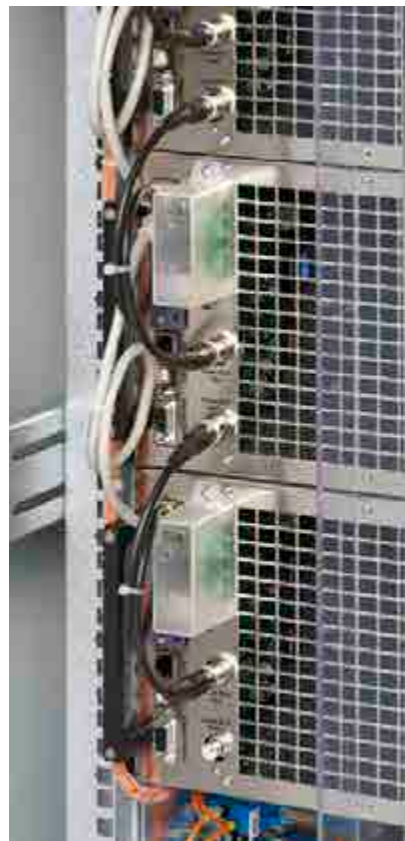
Closeup of Share bus and master-slave bus
