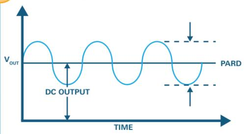
PARD (periodic and random deviation) is the deviation of the DC output from its desired value. It is typically measured in peak-to-peak.
