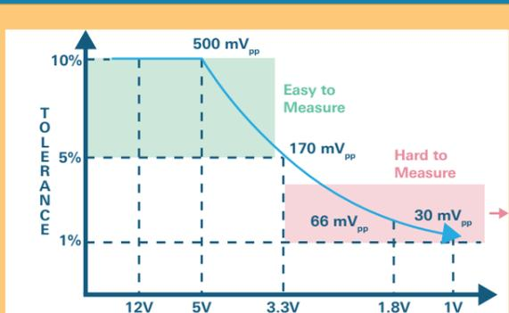
Today's highly integrated electronic devices use smaller voltage levels requiring smaller ripple levels on the power rails for reliable operation. The challenge lies in accurately measuring very small mV level signals riding on power rails.
