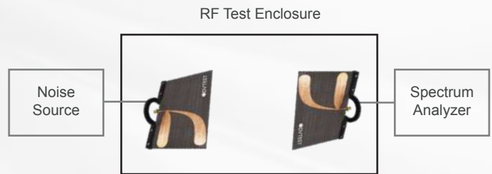
Image 1 Antenna test setup within an RF test enclosure - schematic representation
