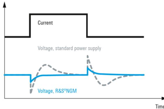
Under challenging load conditions, most power supplies respond with slow recovery times and overshoots. Specially developed circuits in the R&S®NGM200 power supplies achieve a load recovery time of < 30 µs with minimal overshoot, making them perfect for supplying sensitive components.
