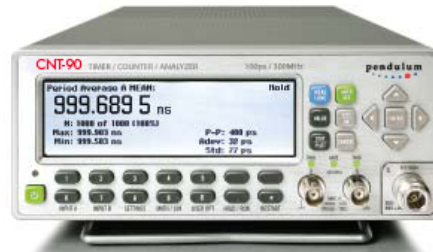
Figure 4: Display showing different statistical parameters viewed at the same time.
