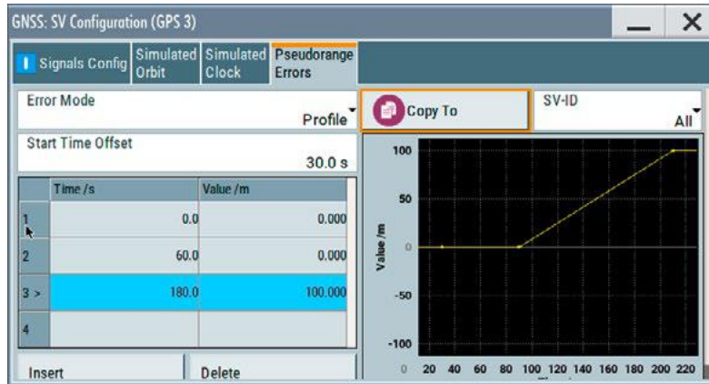
Simulation of a pseudorange ramp for SV 3 with the R&S®SMBV100B for testing the RAIM capabilities of a GNSS receiver
