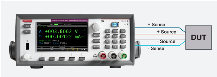
Series 2280S using rear output connector with remote sensing
