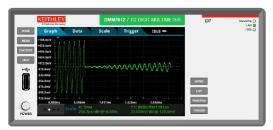
Use the virtual front panel to obtain a full screen display of a waveform. Apply cursors and statistics for waveform analysis.
