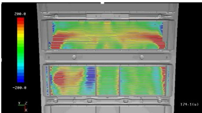
The high definition strain data can be mapped to a 3D CAD model using Luna's 3D visualization tool. Using this tool, engineers can record data during structural testing and then replay the data superimposed on a CAD model of the structure under test. The 3D visualization tool is ideal for problem solving as well as creating presentation materials for management design reviews.
