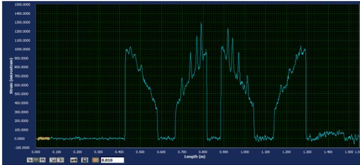
The strain gages can be defined and data displayed using a PC tool. Strain data can be displayed versus the length of fiber or select points can be displayed as a function of time. The PC tool can be used to redefine the strain gage length, the number of data points acquired and the position along the fiber sensor. Data can be acquired over the full length of fiber or from select segments.
