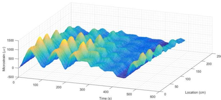
High definition strain data can be stored in a tab delimited text file for exporting to MS Excel or other 3<sup>rd</sup> party analysis software such as Matlab. The high definition data is sufficiently dense to provide a fully contoured view of the strain profile of a structure under load.
